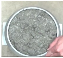
After Rodding 25 times After Tapping 10-15 times Consolidated
