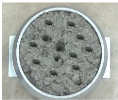
After Rodding 25 times After Tapping 10-15 times Consolidated
